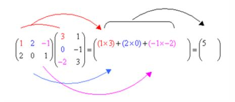
Step 2: Multiply the elements in the first row of A with the corresponding elements in the second column of B. Add the products to get the element C  $_{12}$
